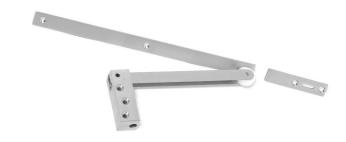
Briton Door Coordinators are designed for use on pairs of doors, where the inactive is requried to close before the active leaf. The door selector is suitable for double rebated doors and fire doors. Door coordination is a basic requirement for all self-closing pairs of doors that are rebated or have astragals.
